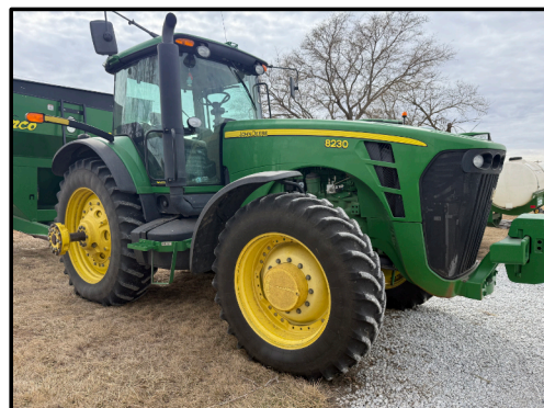
2008 JD 8230 MFWD, 7695 hrs, PS, 4 Hyd, Pwr beyond, w/ quick hitch, 480-80R46 duals SN: RW8230PO23454
